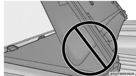
Incorrect Folding – Will Cause Damage
