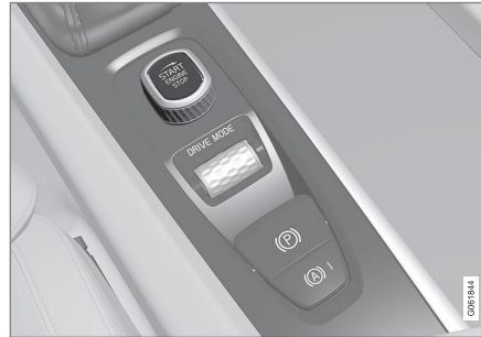
Start knob in the tunnel console.
