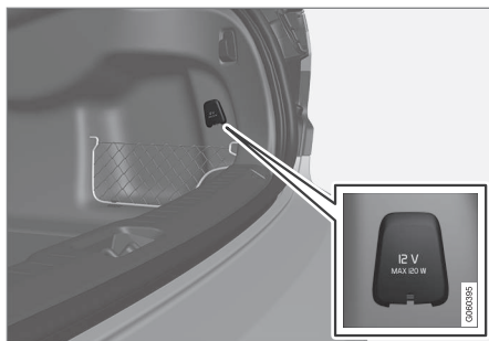
12 V electrical socket in cargo area*.
